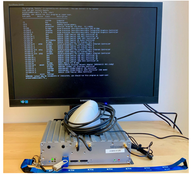
Fig. 7. Nexcom vehicular OBU box [41].
