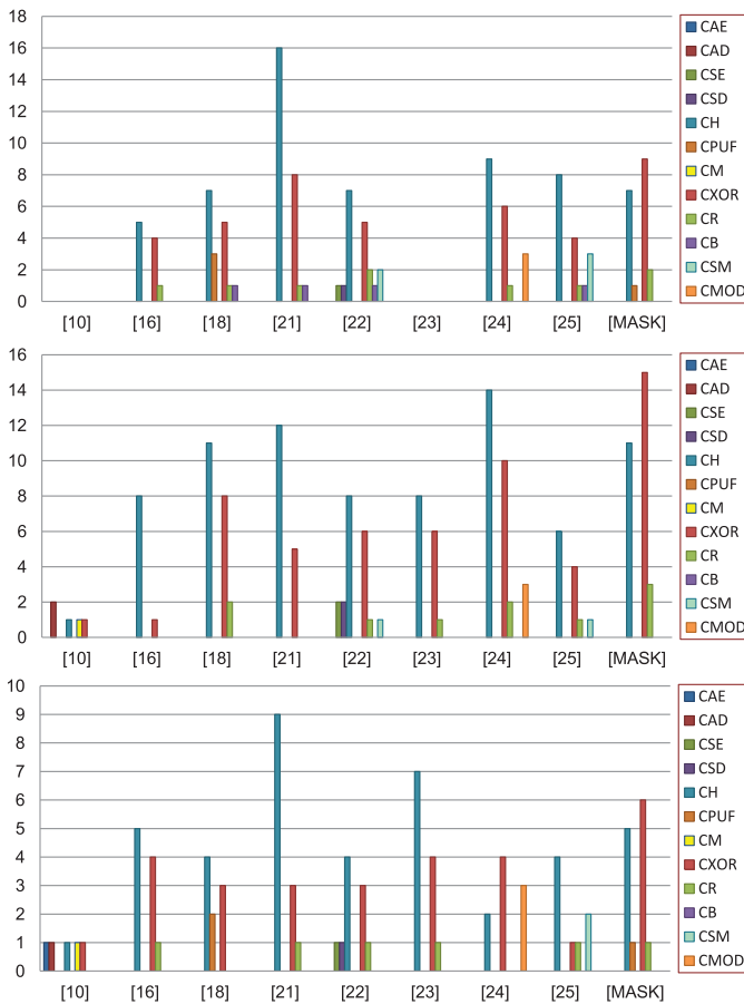
Fig. 7. Computation cost of user (topmost), gateway (middle), and sensor node (bottom-most) of MASK protocol versus conventional protocols.
