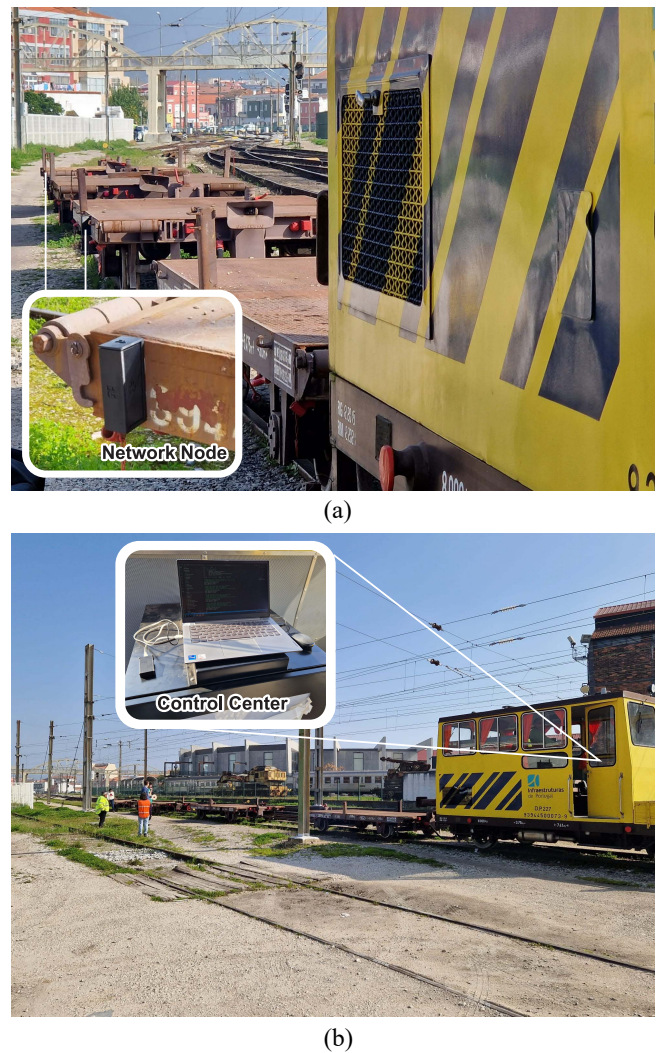
Fig. 21. Field Setup for the train integrity and monitoring system test. (a) Network Nodes placed along the train composition. (b) Network Control Center over the draisine.
