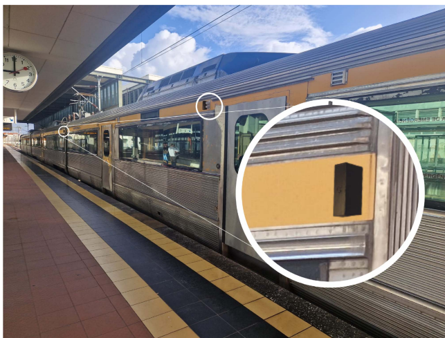
Fig. 20. WSN setup—outdoor train composition test.
