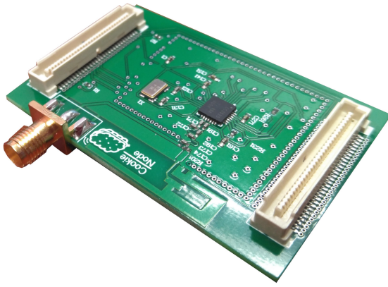
Fig. 1. CC2520-based cookie hardware layer used for the Grey-FTPC implementation.
