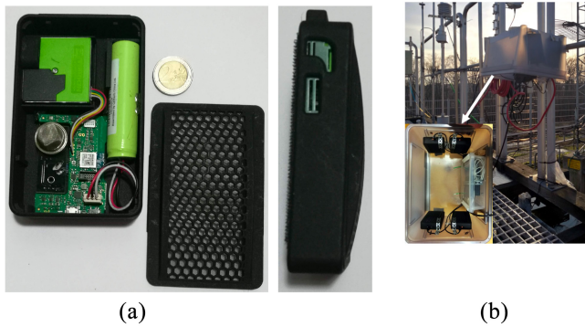
Fig. 1. Sensing systems used in our experiment. (a) Portable LCPs. (b) Installation of four LCPs on SMEAR III under a rain cover.
