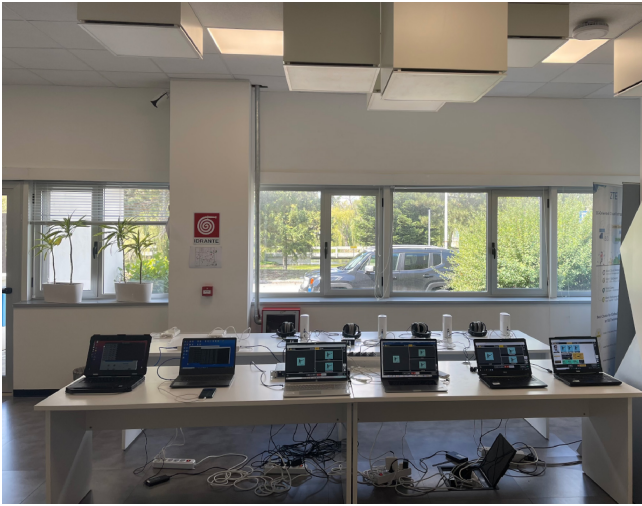
Fig. 3. Picture of the setup of the 5G SA architecture, showing the base station, the six CPEs, the four NMP devices, the four headphones, the sound card, the six laptops, and the smartphone.
