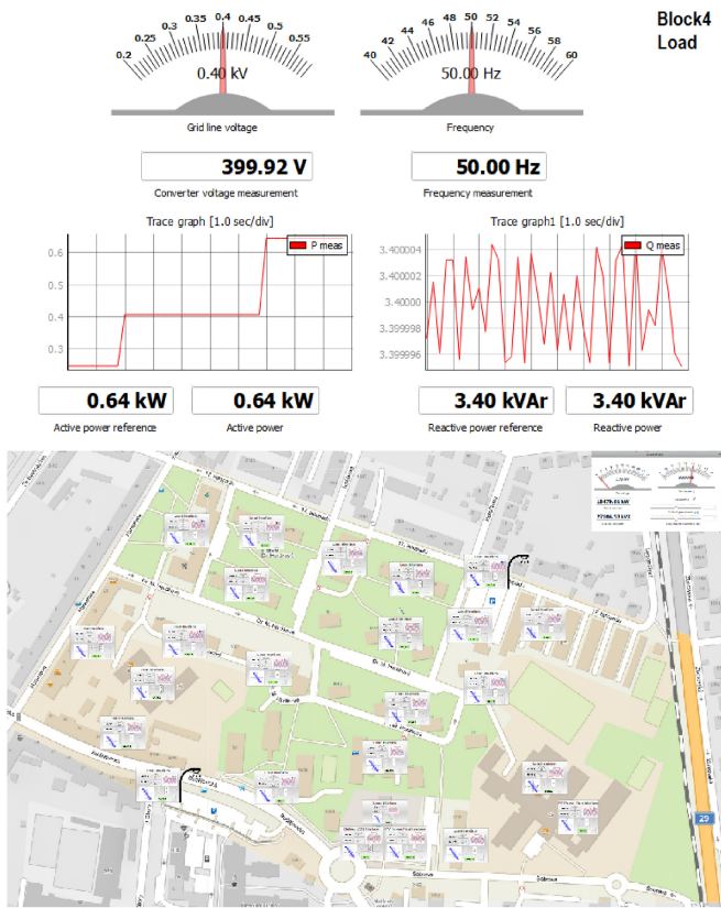
Fig. 5. Simulation of the overall consumption in a PED running in the Typhoon HIL environment. Overview map in the HIL SCADA environment is shown (bottom) with the available controls allowing access to the details of the power consumption and setup of individual parts (top).
