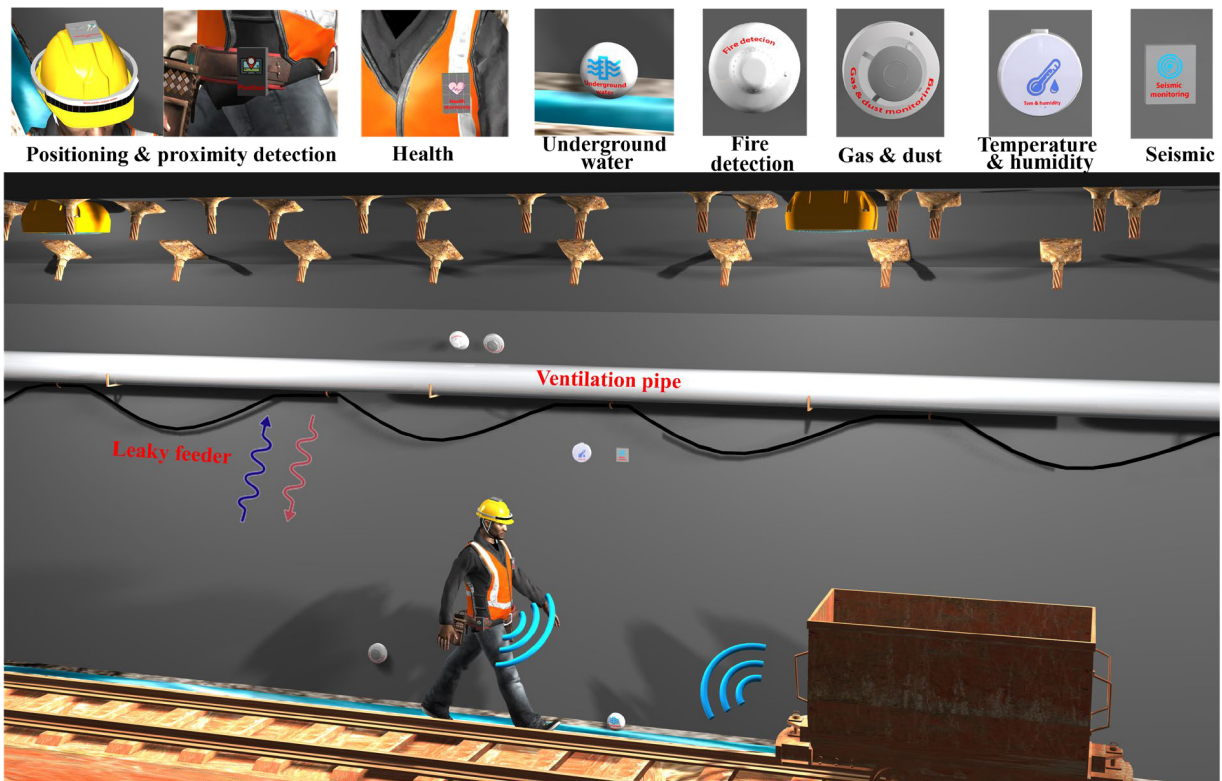
Fig. 3. Sensors used in underground mines for environmental, safety, and production monitoring.
