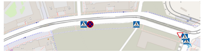
Fig. 16. Detected and localized traffic signs of the real-time layer along the residential area.
