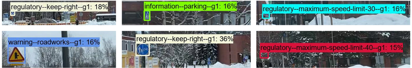
Fig. 9. Examples of mistakes in the objection detection algorithm. On the first row, informative traffic signs of pedestrians crossing are mistaken as being of another type. On the second row, a few more examples of misclassification including an instance where tree branches are mistaken as a traffic sign.
