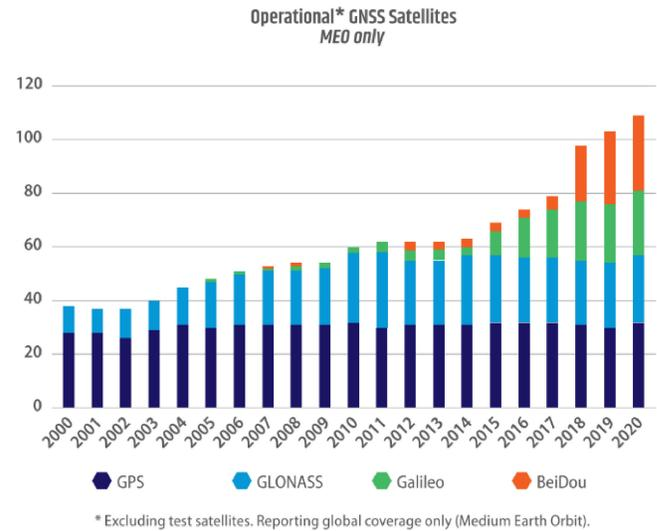
Fig. 14. Evolution of number and distribution of operational GNSS satellites [43].
