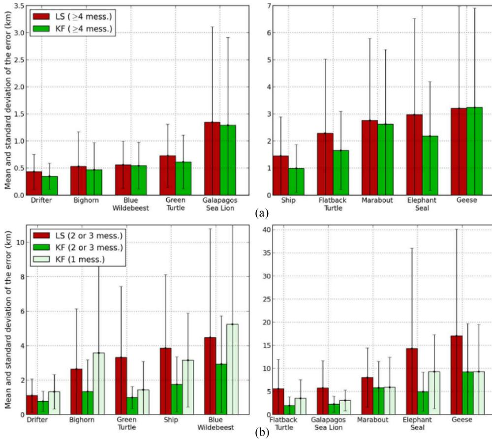
Fig. 12. Mean and standard deviation errors for the Argos LS and EKF algorithms in different tracking uses cases (a) with at least four messages (b) with less than four messages [26].
