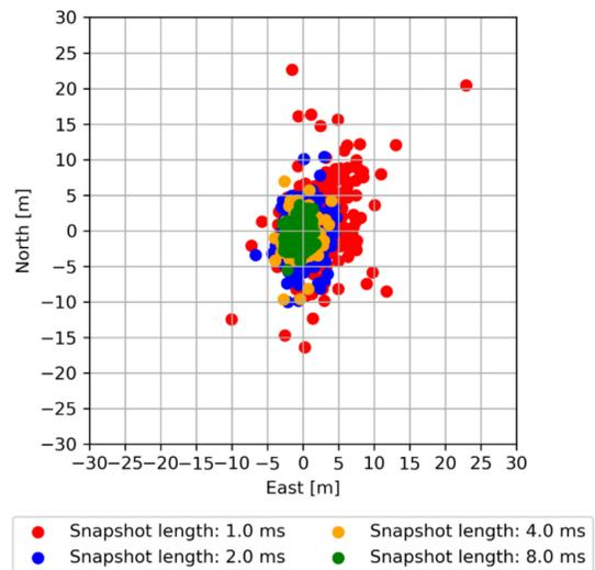
Fig. 9. Time free pseudorange positioning results for various snapshot lengths, using GPS, Galileo, and BeiDou signals [56].
