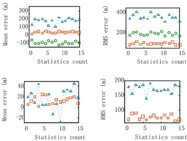
Fig. 11. Mean and RMS errors of east (blue), north (red), and up (green) directions. Top: instantaneous Doppler positioning. Bottom: height aiding [31].
