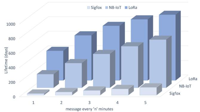
Fig. 4. Battery lifetime for different LPWAN technologies and uplink message update rates, using a 5-byte payload size and a 2500-mAh battery [40].
