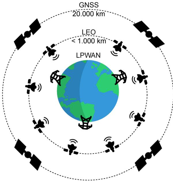
Fig. 1. Three categories of technologies enabling large-scale positioning. The ground segment of the satellite systems is not shown.
