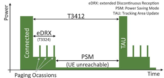
Fig. 5. NB-IoT transmission cycle with sleep mechanisms [41].
