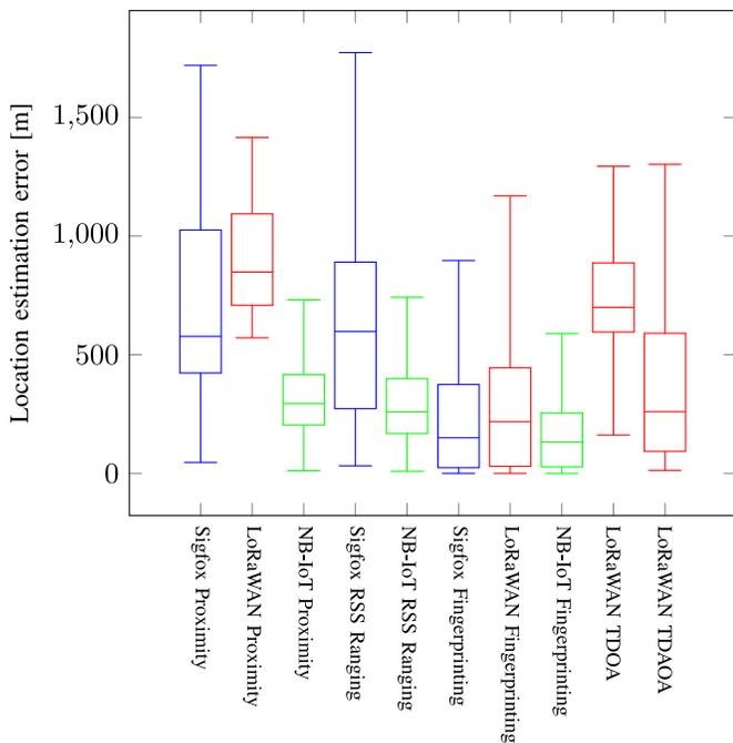
Fig. 8. Positioning accuracy of LPWAN localization algorithms [13], [14], [15], [19].
