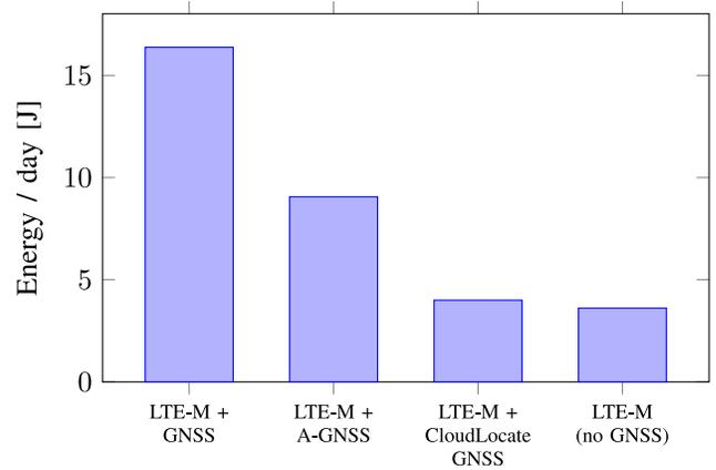
Fig. 6. Total daily energy consumption comparison of different GNSS techniques, for a UE combining a u-blox M10 chip with LTE-M connection, with six location updates per day [48].
