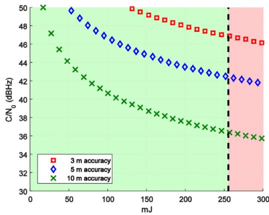
Fig. 10. Expected energy consumption and accuracy of a cloud-based GNSS sensor under different  $C/N_0$  environments [35].
