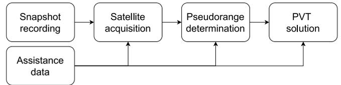
Fig. 3. Block diagram of snapshot processing using GNSS. Note that all steps except the snapshot recording might be outsourced from the UE to the cloud.
