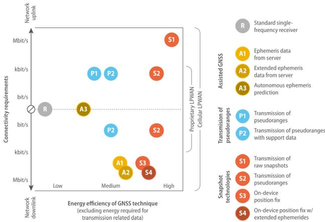
Fig. 7. Relationship between connectivity requirements and energy efficiency of different GNSS techniques [49].
