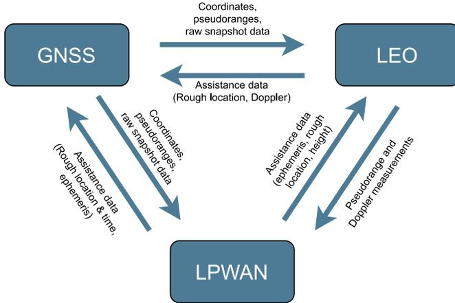
Fig. 18. Interoperability of LPWAN, GNSS, and LEO positioning systems.
