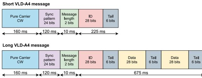
Fig. 17. Message structure of the Argos VLD-A4 transmission standard.
