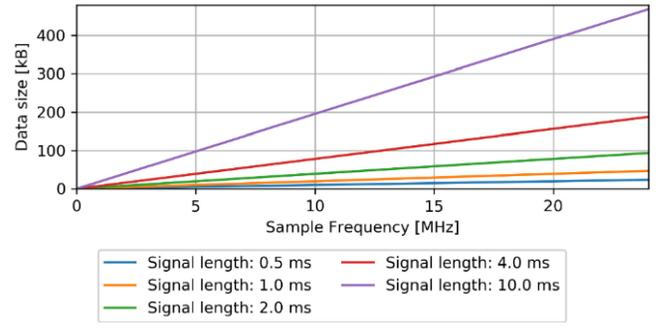
Fig. 16. Relationship between snapshot length, sampling frequency, and snapshot size for an 8-bit quantization [56].
