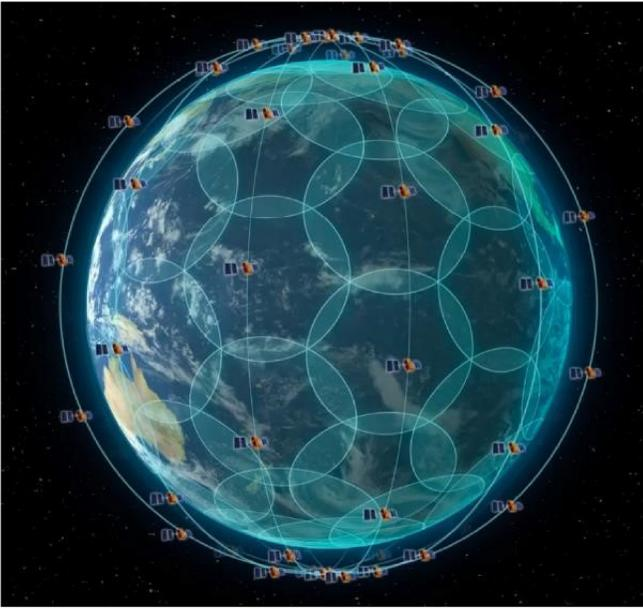
Fig. 15. 66 LEO satellites of the Iridium NEXT constellation with their footprints on Earth [64].
