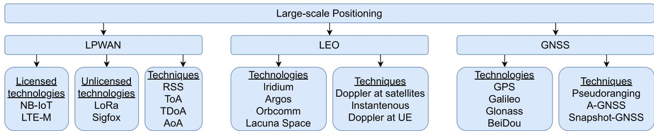
Fig. 2. Overview of large-scale positioning technologies and techniques discussed in this work.
