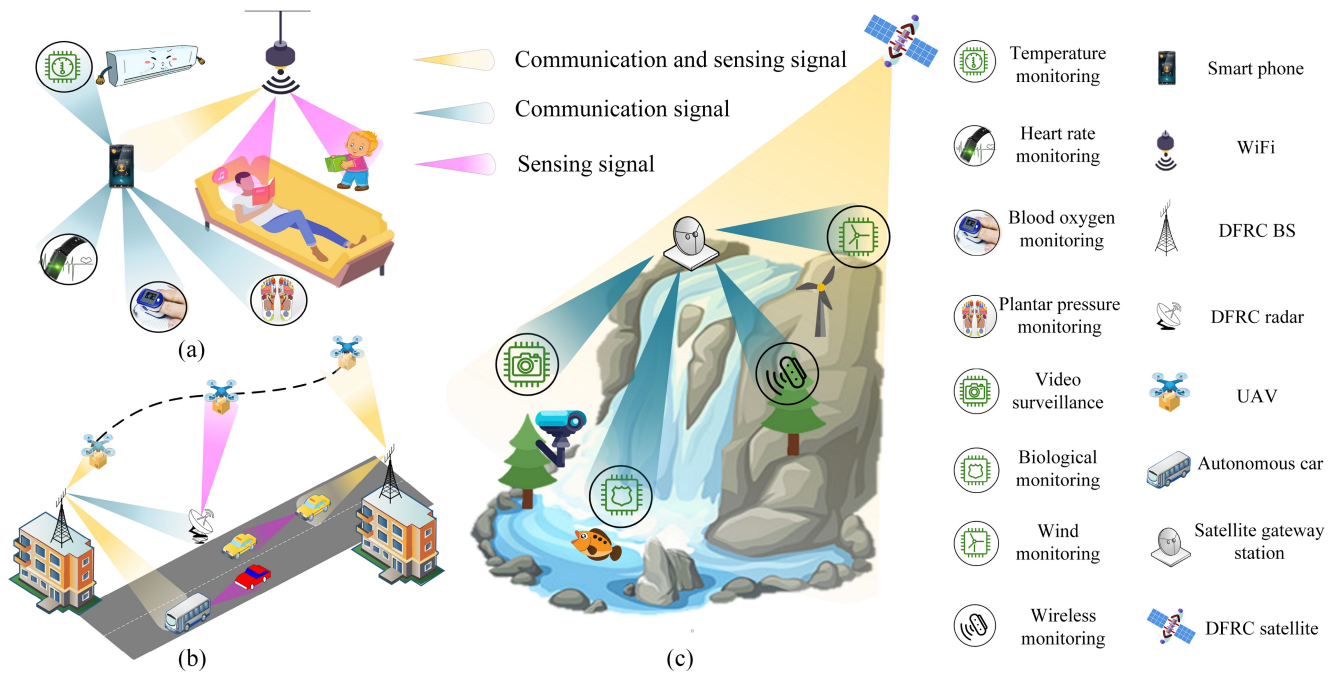
Fig. 8. Illustration of the three typical applications of JCAS in IoT, i.e., (a) smart home, (b) autonomous driving, and (c) delivery and environmental monitoring.
