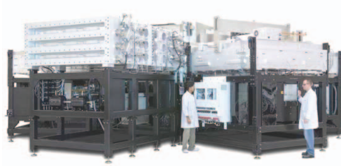
Figure14. 8.5 th -Generation CVD system (courtesy of AKT)
