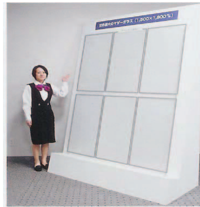
Figure12 6 th -Generation glass can have six 32-in. LCD substrates.
