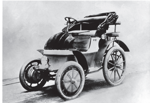
Figure 8. Ferdinand Porsche's electric car of 1899, with hub-motor at each driving wheel (source: http://stuttcars.com )
