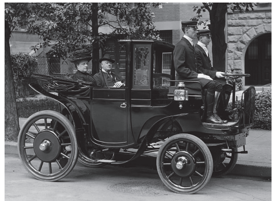
Figure 6. A France made Krieger electric landaulet in Washington, D.C., circa 1906, owned by senator George P. Wetmore (Courtesy of Library of Congress, Prints & Photographs Division.)
