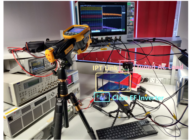
Fig. 21. Photograph of the final experimental setup during operation connected to the oscilloscope for performance verification. The individual parts of the system are highlighted accordingly.
