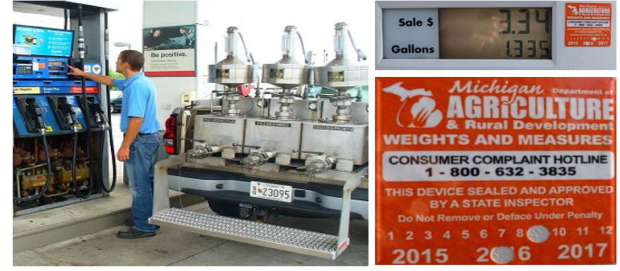
Fig. 3. U.S. Weights and Measure Program qualifies secured gas pump metering (left) with a seal (right). [Photo (left): Weights and Measures, Maryland Department of Agriculture].
