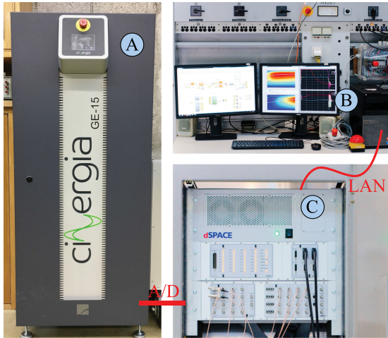
Fig. 6. Laboratory setup. (a) Cinergia grid emulator. (b) Host-PC. (c) dSPACE real-time system.
