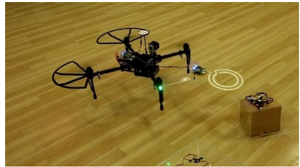
Fig. 17. Photograph of the wireless charging drone.
