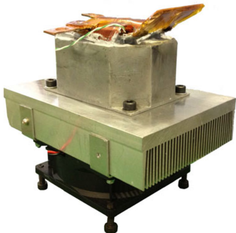
Fig. 10. Potted inductor on a heat sink with fan, thermal insulation not shown.
