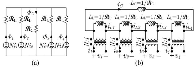
Fig. 12. (a) Reluctance model for the four-phase coupled inductor geometry presented in Fig. 8.  $\mathcal{R}_L$  represents the reluctance of the path the flux takes through the bottom plate, post, and top plate, for one of the phases.  $\mathcal{R}_C$  represents the leakage path through the air gap in between the top and bottom plates. (b) Inductance dual model representation of the reluctance model, obtained by taking the topological dual.
