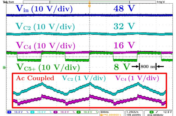
Fig. 21. Measured waveforms of the input voltage, differential voltage across  $C_2$  and  $C_4$ , and switch node voltage  $V_{C5+}$  (labeled on Fig. 4) during 48 to 1 V operation at an output current of 240 A. The SC stage is switching at 432.9 kHz. The AC coupled waveforms of  $V_{C2}$  and  $V_{C4}$  highlight that the flying capacitors are being soft-charged by the inductor current in the multiphase buck stage.
