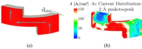
Fig. 14. (a) Approximation of the ac winding resistance for the vertical coupled inductor structure in Fig. 16 used in the optimization to compute the ac winding loss. It is assumed that the ac current only flows through the outer surface of the conductor. (b) ANSYS Maxwell 3D Eddy Current simulation of the current density distribution of one of the windings. Each winding is excited with a sinusoidal ac current of 2 A peak-to-peak at a frequency of 1.5 MHz.
