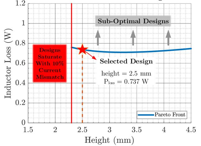
Fig. 15. Results of the optimization routine for the vertical coupled inductor showing the Pareto front of the inductor loss versus its height. The optimization is performed at a dc current of 20 A per phase and a switching frequency of 1.5 MHz. The selected height of the vertical coupled inductor for Mini-LEGO is 2.5 mm, resulting in an estimated loss of 0.737 W at full load.
