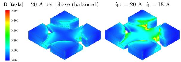
Fig. 18. Magnetostatic finite-element simulation (ANSYS Maxwell 3D) of the designed coupled inductor. The simulation was conducted both under balanced DC phase currents equal to 20 A per-phase (left) and a phase current imbalance of 10% (right) where three phases are carrying 20 A of current, while the fourth is carrying 18 A. The peak flux density of the core is 190 mT in the balanced condition and 390 mT in the imbalanced condition.
