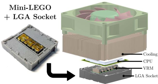
Fig. 2. VRM placed within a modified LGA socket (Intel LGA1155) for CPUs. Copackaging the VRM inside the LGA socket can leverage the cooling resources of the CPU and perform point-of-load power delivery. The VRM must have small enough area and thin enough height.
