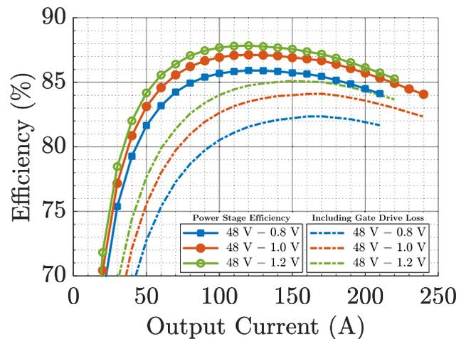
Fig. 26. Measured efficiency of the Mini-LEGO converter with and without gate driving losses during 48 to 0.8 V, 1.0 V, and 1.2 V conversion. For 48 to 1 V, without the gate driving losses, the Mini-LEGO converter achieves a peak efficiency of 87.1% at 120 A and a full load efficiency of 84.1% at 240 A.
