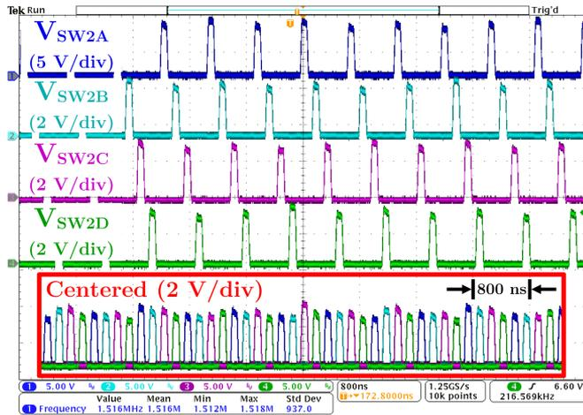
Fig. 23. Measured waveforms of the switch node voltages in the second submodule of the multiphase buck stage ( $f_s = 1.515$  MHz) during 48 to 1 V operation at an output current of 240 A. The input voltage of the second submodule of the multiphase buck stage is equal to  $V_{BUS2}$ .
