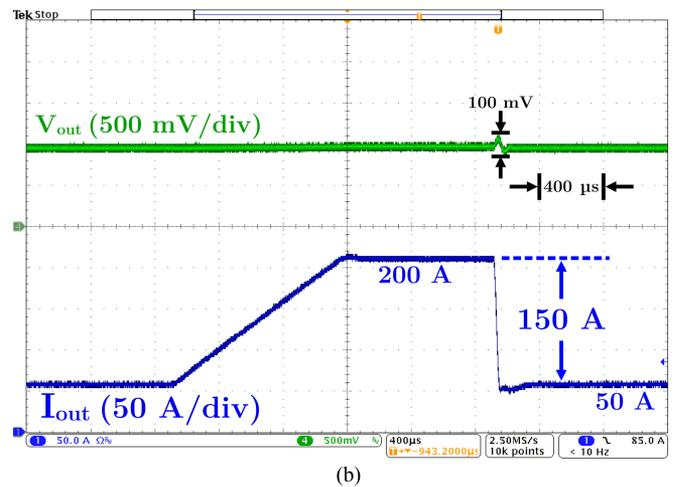
Fig. 25. Measured waveforms during a load current transient from 50 to 200 A to 50 A (62.5% load step) of (a) the three intermediate bus voltages, and (b) the output voltage during 48 to 1 V operation. A voltage-mode control method was implemented using a TMS320F28388D microcontroller. The output capacitance is 2.5 mF.
