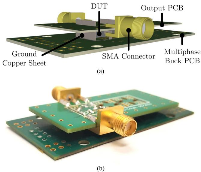
Fig. 32. (a) Altium 3-D Rendering of the test fixture assembly and (b) fully assembled test fixture with DUT in place. The DUT is connected to the multiphase buck board used in the Mini-LEGO converter. An output board is designed and connected to the DUT and ground copper sheets. Two SMA connectors are placed on the output board and used to interface with the VNA to conduct the measurements.
