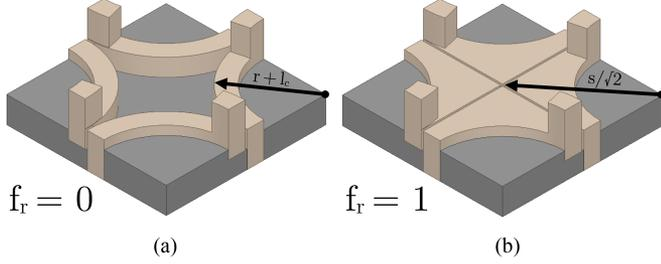
Fig. 11. Winding fill factor parameter  $f_r$  at (a) its minimum condition of  $f_r = 0$  and (b) its maximum condition at  $f_r = 1$ . The fill factor parameter is independent of the core geometry and can be used to further fine tune the per-phase transient inductance and DC resistance of the coupled inductor after the core is manufactured.
