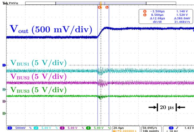
Fig. 24. Measured waveforms of the output voltage and three virtual intermediate bus voltages in response to an open-loop duty cycle transient from 15% to 20% during 48 to 1 V operation at an output current of 120 A. The output voltage changes from 1.14 V to within 2% of the new output voltage of 1.5 V within 12  $\mu$ s. The output capacitance is 2.5 mF.
