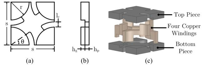
Fig. 8. (a) Top view and (b) side view of the vertical coupled inductor structure highlighting the geometric parameters used for optimization. (c) Vertical coupled inductor two-piece assembly, illustrating the copper winding positioning between the top and bottom magnetic core pieces.
