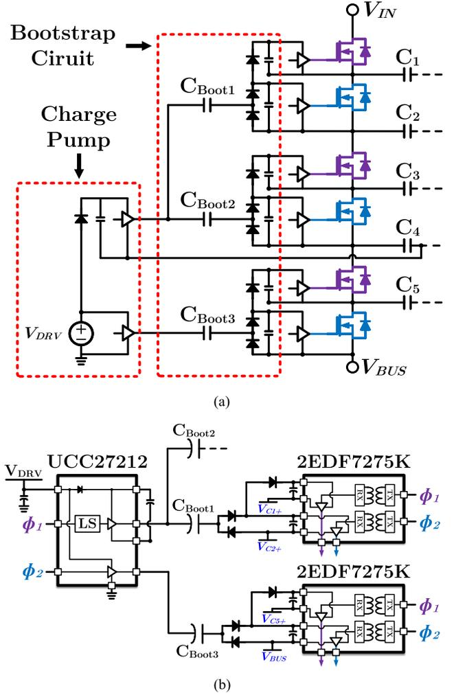
Fig. 6. (a) Circuit schematic of the gate drive for the floating switches of the SC stage. (b) Implementation of the charge pump, bootstrapping circuit, and gate drivers. An isolated gate driver IC (2EDF7275 K from Infineon) is used to drive each of the floating dual-channel MOSFETs.
