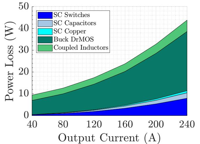
Fig. 29. Calculated loss breakdown of the Mini-LEGO converter during 48 to 1 V operation. The SC stage loss is split into switching and conduction losses due to the switches, energy and conduction losses due to the capacitors, and loss due to the PCB and vertical copper connectors. In the multiphase buck stage, the loss is divided into the device switching and conduction losses and the winding and core losses from the coupled inductors.
