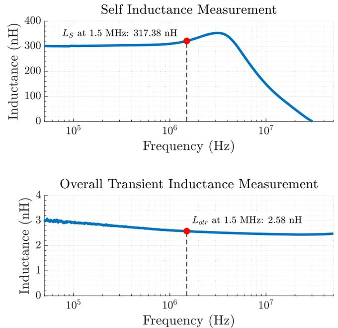
Fig. 33. Measured data of the self inductance (top) and overall transient inductance (bottom) of the vertical coupled inductor. The self inductance is 317.38 nH at 1.5 MHz, and the overall transient inductance is 2.58 nH at 1.5 MHz. The measurements include parasitic inductances of PCBs and GND copper sheets on paths.
