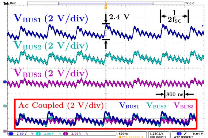
Fig. 22. Measured waveforms of the three virtual intermediate bus voltages during 48 to 1 V operation at an output current of 240 A.  $V_{BUS1}$  has the highest peak-to-peak voltage ripple at 2.4 V, since flying capacitors  $C_1$  and  $C_2$  have the lowest effective capacitance. The ripple frequency of the intermediate bus voltage is equal to twice the switching frequency of the SC stage (432.9 kHz). All three intermediate bus voltages are balanced at 8 V.
