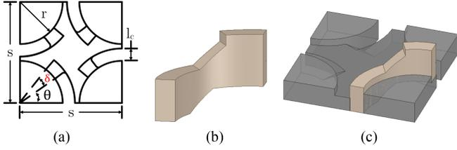
Fig. 10. (a) Top view of vertical coupled inductor structure with the addition of  $\delta$ . (b) Winding design, with angled copper for continuous conduction path. (c) Winding placement within the magnetic core.
