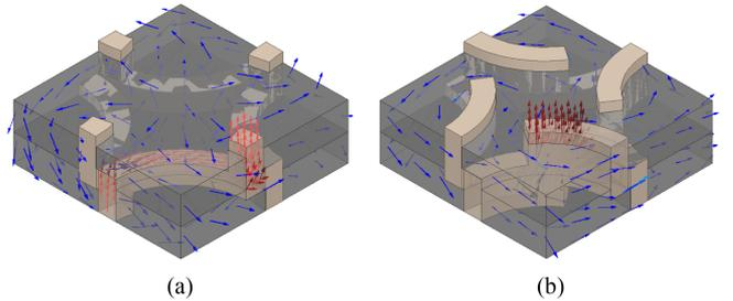
Fig. 9. Demonstration, using ANSYS Maxwell 3D, of how varying  $\theta$  impacts the current and flux distribution for (a)  $\theta = 15^\circ$  and (b)  $\theta = 57^\circ$ . The blue arrows on the magnetic core pieces show the flux density, and the red arrows on the winding show the current density.
