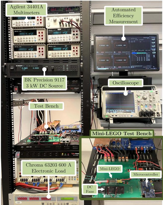
Fig. 20. Experimental test setup for characterizing converter performance. The Mini-LEGO converter is connected to an output motherboard that hosts the fans and interfaces with a DC source, microcontroller, and electronic load.
