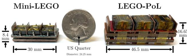
Fig. 3. Side-by-side comparison of the Mini-LEGO prototype presented in this article (developed in 2023), the vertical stacked LEGO-PoL prototype presented in [13] (developed in 2021), and a United States quarter. The volume of the 240 A Mini-LEGO is 22.5% of the 450 A LEGO-PoL. The height is reduced from 16.65 to 8.4 mm, and the area is reduced from 767 to 336 mm<sup>2</sup>. It took 24 months to increase the power density two times.
