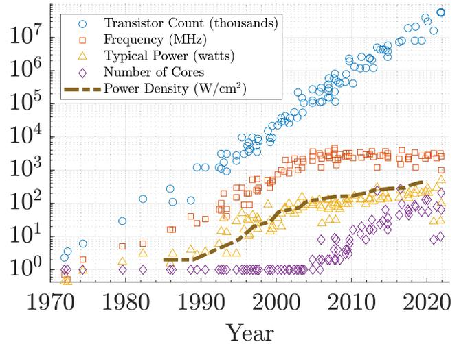
Fig. 1. Microprocessor trend data over the past 50 years (reproduced with data from [6], [7]). The transistor count per area doubles every 18 months (Moore's Law). As Dennard scaling has broken down, microprocessors have shifted to multicore systems to keep increasing transistor count year after year [8]. The increased power consumption per square centimeter of microprocessors requires dense and efficient voltage regulators.
