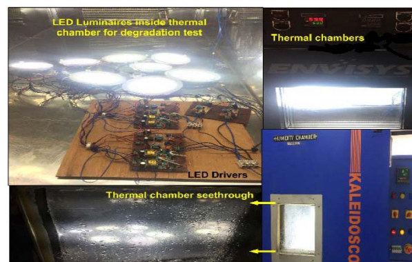
FIGURE 4. The electrical and optical characteristics measurement set-up during ADTS1/ADTS2 conditions.
