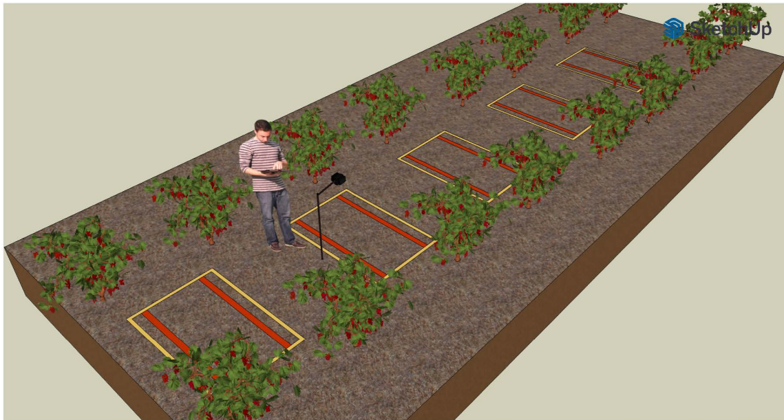
FIGURE 4. Layout of terrain surveys. In yellow the camera acquisition frames, in red the profile sampled with the roller chain and pin meter.
