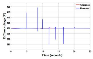
FIGURE 14. The DC bus voltage results.
