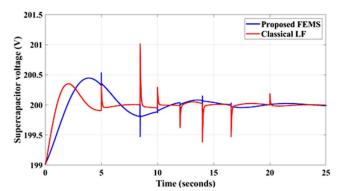
FIGURE 16. The supercapacitor voltage results for the proposed and LF strategies.
