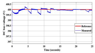
FIGURE 7. The DC bus voltage results.
