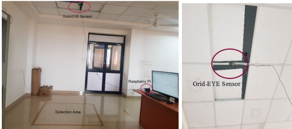
FIGURE 15. Data acquisition setup.
