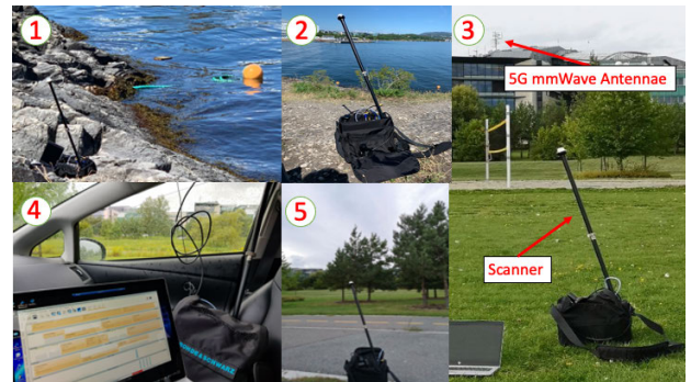
FIGURE 2. Some measurement locations: 1) close to water, 2) 6 m above water, 3) Line of Sight, 4) rain, 5) foliage blockage.
