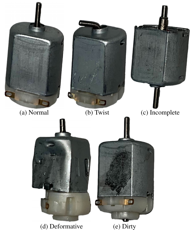
FIGURE 6. The data samples of the Industrial Part Defect Dataset. The normal target is the normal status of the industrial part, the others represent 4 abnormal status.
