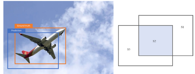
FIGURE 7. IoU calculation diagram. The Ground truth box is the true label of the target like the S1, the prediction box is the output prediction from model like the S3, the overlapping area is the S2, and the IoU is calculated by the S1, S2 and S3.
