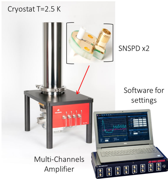
FIGURE 8. SNSPD detector bundle from Single Quantum B.V. The two SNSPDs are in the cryostat, which is the red box with the gray tower, the RF amplifiers are in the black box, and the PC is used to set the bias and monitor the DCR and SDE.
