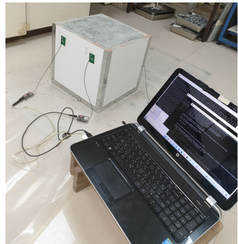
FIGURE 7. Water content and compaction estimation experiments.
