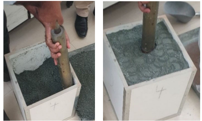
FIGURE 9. Initial (left) and final (right) compaction stages of dry crushed sand.
