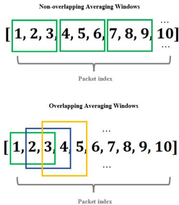
FIGURE 1. Comparison between non-overlapping and overlapping averaging windows. Each number represents a packet.
