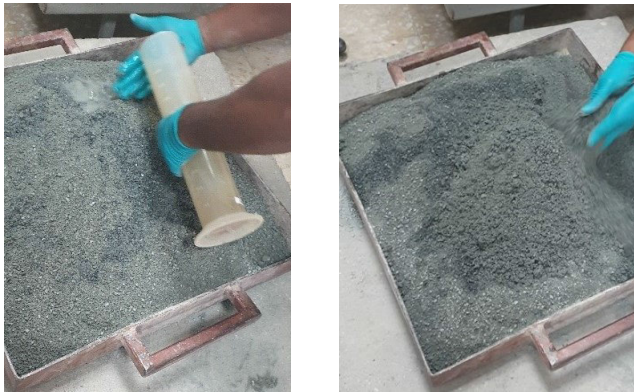
FIGURE 8. Crushed sand addition of water and mixing process.
