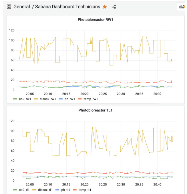
FIGURE 4. SABANA Graphics for Technicians. Visualization of two photobioreactors RW1 and TL1.
