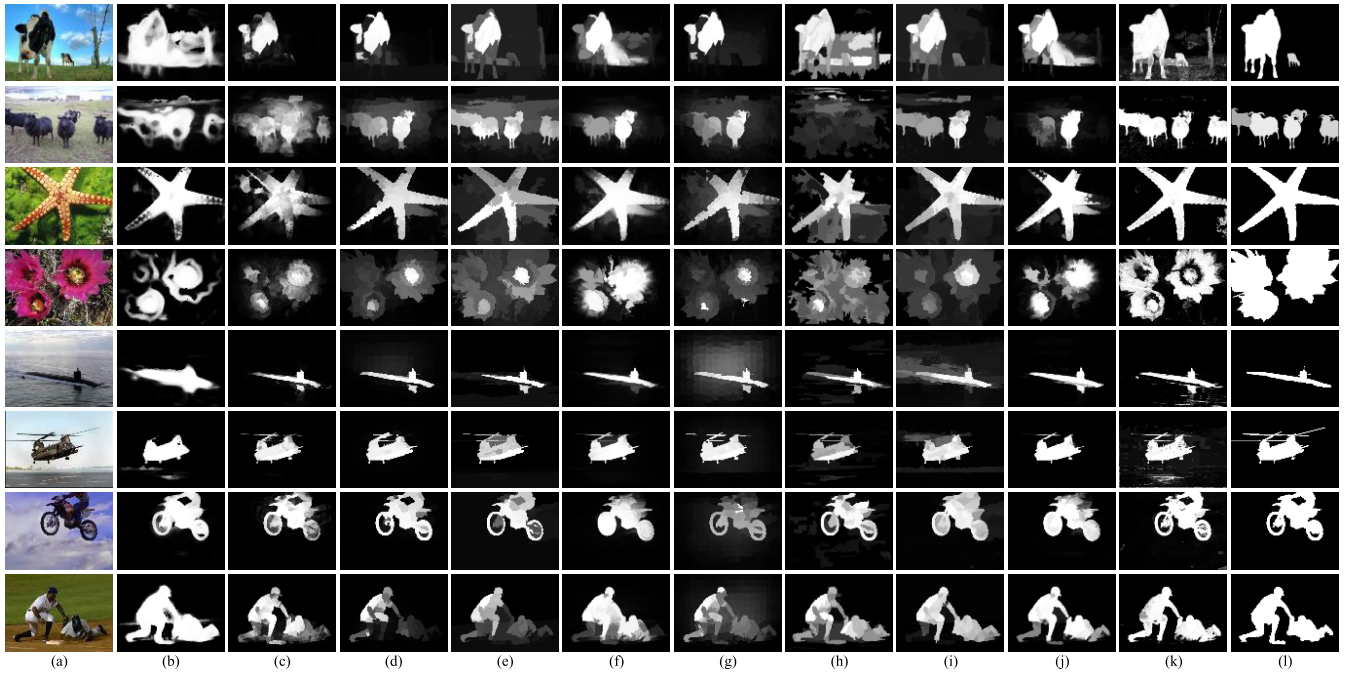
FIGURE 4. Some saliency maps produced by the top-ten performing methods on the four benchmark datasets. Each column from (a) to (l) is respectively the input images, saliency maps of CGVS, DSR, GMR, HS, MBS+, MC, RC, ST, WF and DML, and the ground truths. Every two rows from top to bottom correspond to sample images from PASCAL-S, ECSSD, DUT-OMRON and THUS-10000 dataset.
