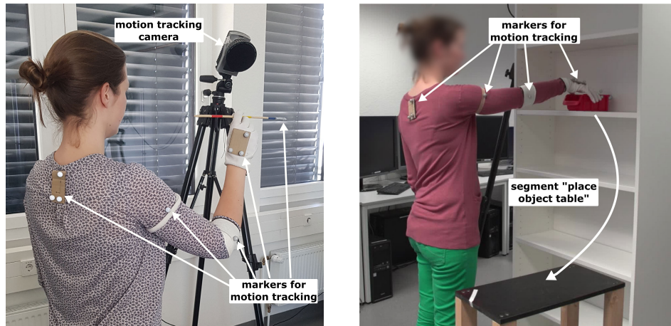
FIGURE 3. Setups for movement recordings. Left: Setup for stick-throwing recordings. (Image extracted from [24].) Right: Pick-and-place task, in which a box is grasped from a shelf, placed on a table, and vice versa. (Image adapted from [25].)
