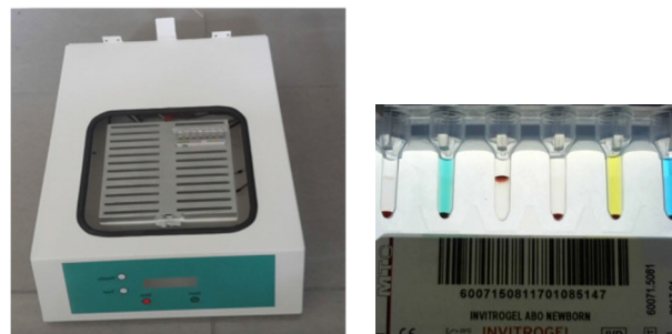
FIGURE 1. The gel card incubator (left) with a gel card (right).
