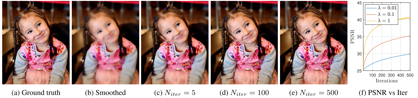
FIGURE 5. Results of reversing a bilateral filter using the TDA-method with \lambda = 1 . (a) Original image. (b) Smoothed image with BF (25.3dB). (c) Result after 5 iterations (29.9dB). (d) Result after 100 iterations (37.0dB). (e) Result after 500 iterations (40.9dB). (f) PSNR as a function of N_{iter} for three settings of \lambda .
