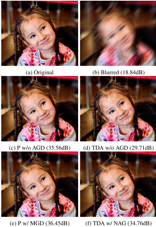
FIGURE 15. Example of reversing a motion blur filter with P-method and TDA-method by applying accelerated gradient descent. (a) Original image. (b) Blurred image. (c) P-method. (d) TDA-method. (e) P-method with MGD. (f) TDA-method with NAG.
