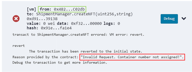
FIGURE 7. Reverted function execution when createNFT() function is invoked prior to shipment approval and container identifier setting.
