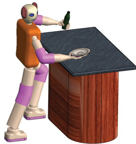
FIGURE 1. Illustration of the hybrid robot built from rigid links and VSPs (pink colored). The VSPs are installed at its feet, knees, elbows, and palms. These are body parts which frequently interact with unknown objects and environment.
