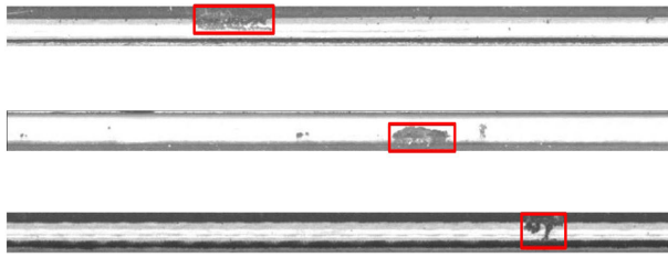
FIGURE 2. Defects combined with rail edges.
