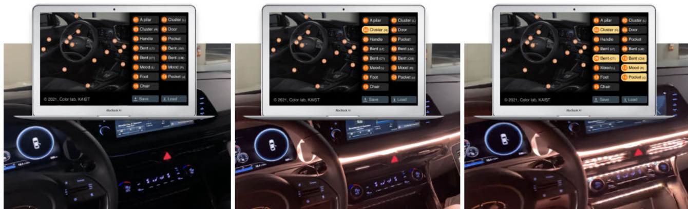
FIGURE 2. Manipulating LED stripes mounted in a passenger car (Sonata DN8, Hyundai Motor Company) using light control software. (left) A control panel contained 15 buttons to switch the light components on or off in 15 regions. (mid) Press button number 3 and turn on the right side of cluster part lighting. (right) Press buttons number 3, 9, 10, 12, and 14 and turn on the lighting of cluster right, bent, mood, and pocket.
