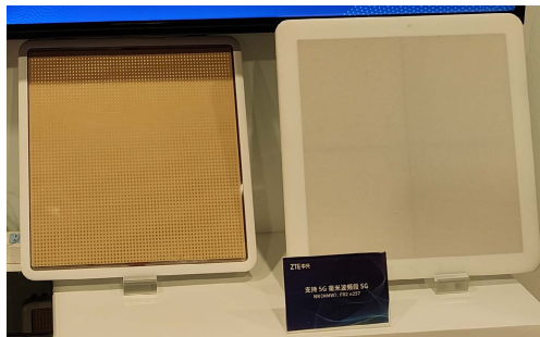
FIGURE 6. Two RISs fabricated for test purposes, the right one with a protecting mask.
