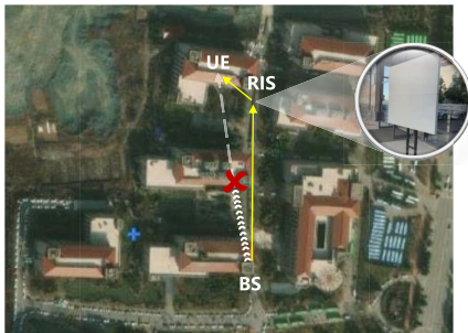
FIGURE 13. Test environment for outdoor to indoor trials at 2.6 GHz.
