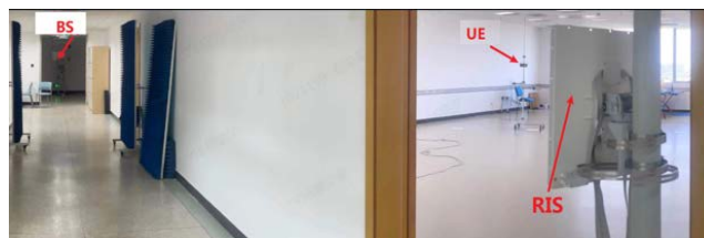
FIGURE 8. Setup for the indoor OTA test.
