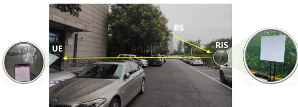
FIGURE 14. Test environment for outdoor to indoor trials at 4.9 GHz.
