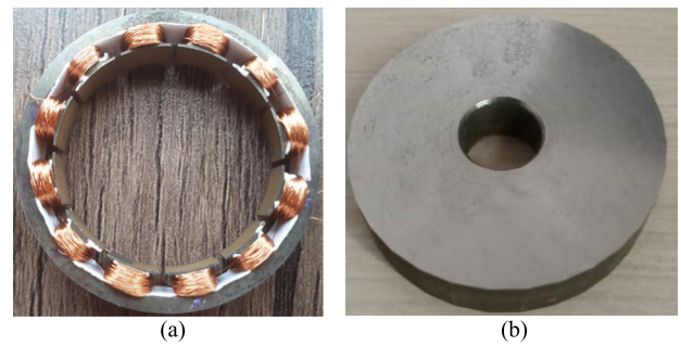
FIGURE 11. Prototype 1-X VR resolver with CTNOW configuration. (a) Stator and (b) Rotor.
