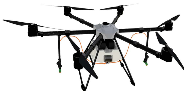
FIGURE 3. Implemented hexacopter drone for spraying fertilizer and pesticides in paddy fields.
