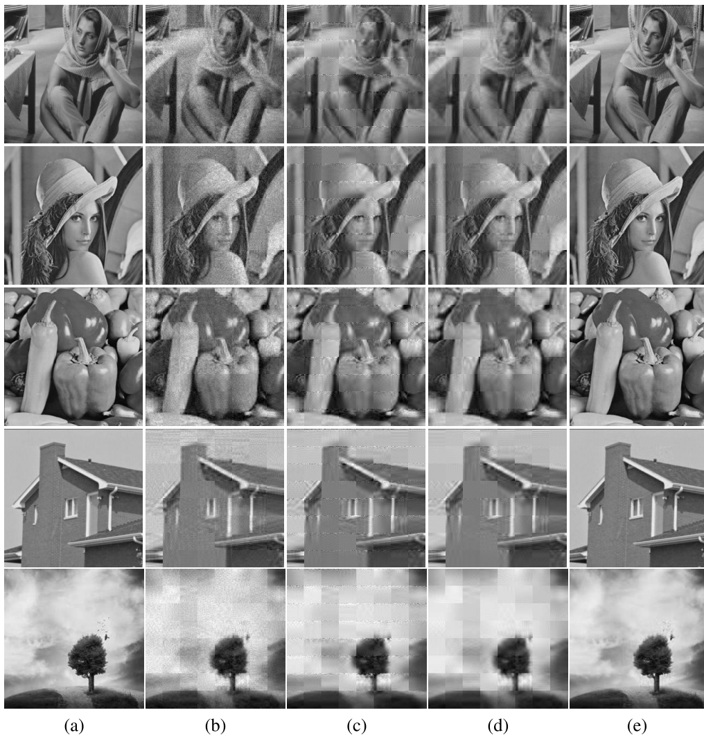
FIGURE 8. The original image and the corresponding recovered results by different algorithms with the sampling rate m/n = 30 . (a) is the original image; (b) shows the result obtained by L1; (c) shows the result obtained by TV; (d) shows the result obtained by L1-TV; (e) shows the result obtained by Adap L1-TV.
