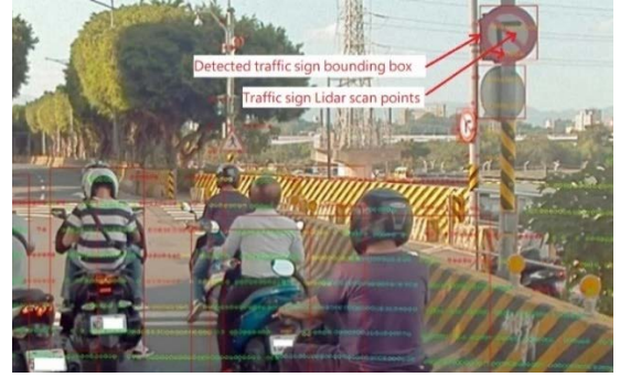
FIGURE 14. Lidar scan points (colored dots) mapped to their corresponding pixels of the detected traffic sign by applying rotation and translation parameters.
