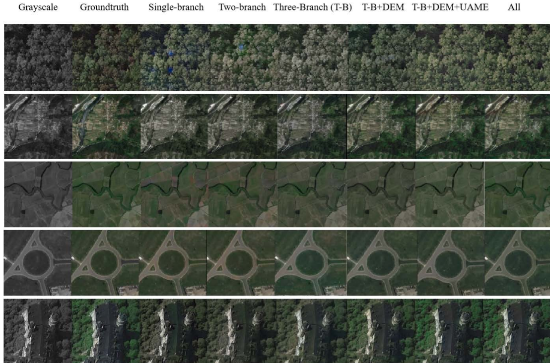
FIGURE 6. The generated images of the ablation experiments. The images generated by the multi-branch structure have stronger spatial consistency than the images generated by the single-branch structure. For example, the first row and the third column of the pictures contain distinguishable blue areas from the surrounding area which disappear in the fifth column. After adding the DME module, the generated images have stronger object salience, such as the image shown in the first row in the sixth column. Inconsistent colors disappear after adding the UAMB module, as shown in the seventh column of the first row, demonstrating the role of this module in enhancing color space consistency. The addition of the MMB module further optimizes the generation results by balancing object salience and spatial consistency, as shown in the first row and the last column.
