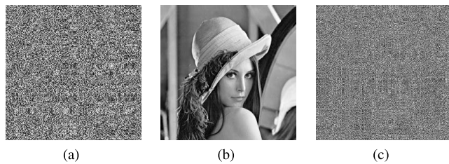
FIGURE 10. Key sensitivity test. (a) cipher image with original key; (b) decryption by original key; (c) decryption by incorrect key.
