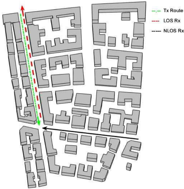
FIGURE 2. Simulation environment with a LOS and NLOS scenario used for data set generation.
