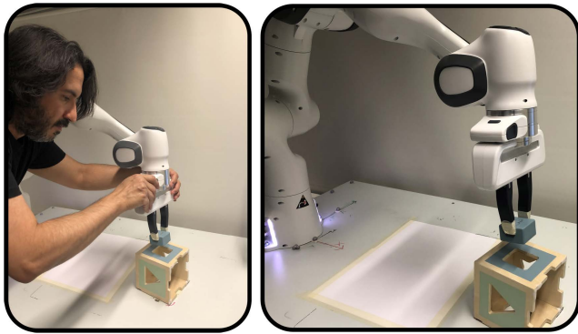
FIGURE 1. Left: A human operator teaches a robot how to perform a PiH task. Right: a snapshot showing the PiH task executed by a Franka Emika Panda robot.
