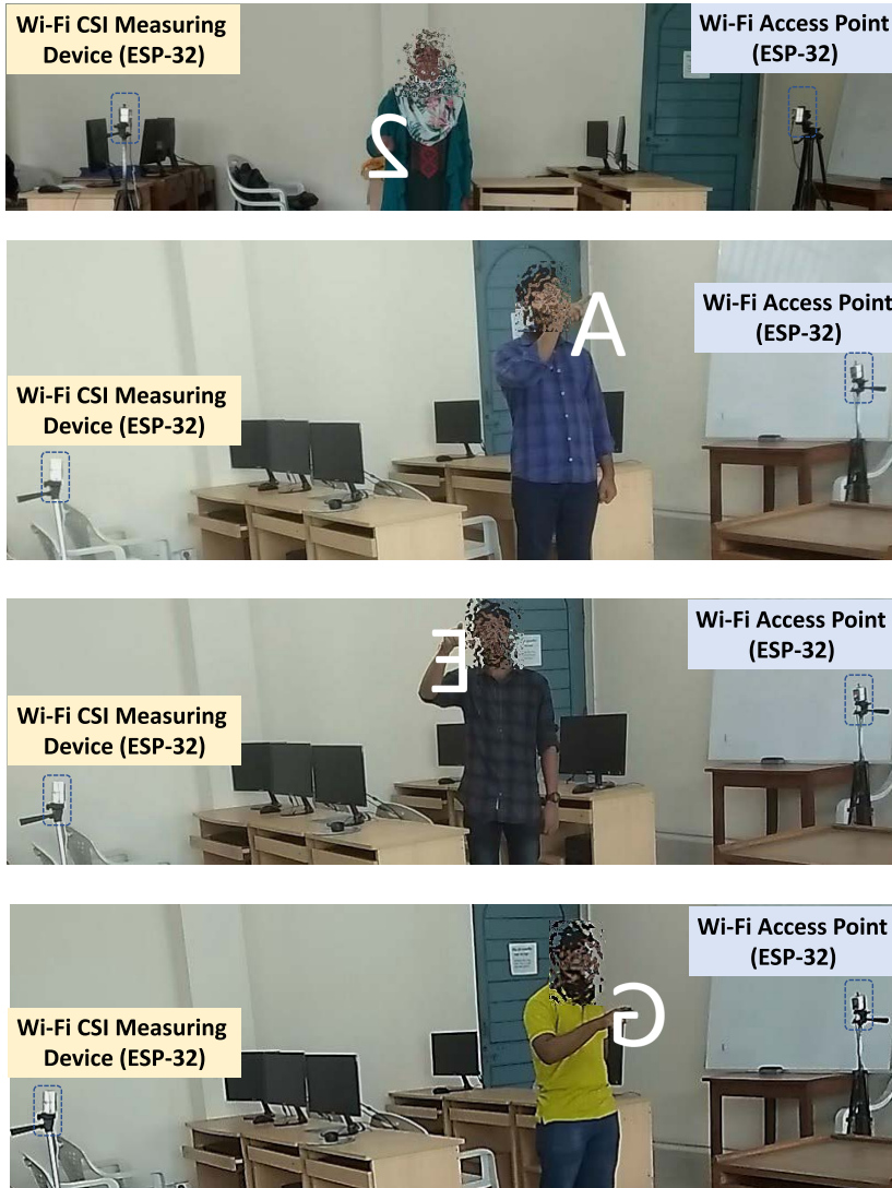
FIGURE 4. Test-bed scenario when the transmitter and receiver are 2 m apart.
