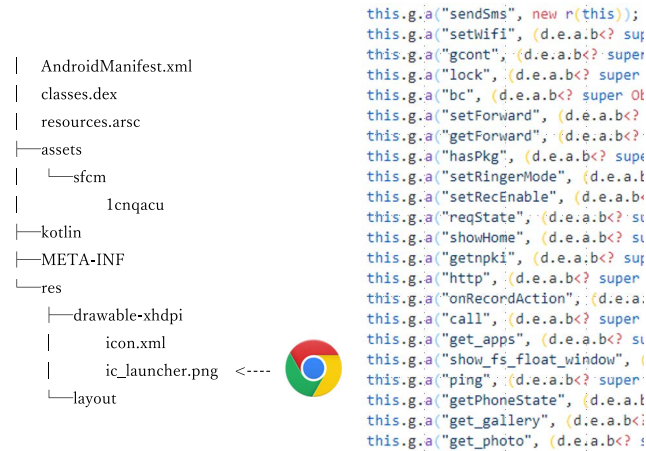
FIGURE 4. (Left) Directories, files, and the malware icon after decompressing Chrome.apk. (Right) Twenty-two C2 commands in the payload defined as Java methods.
