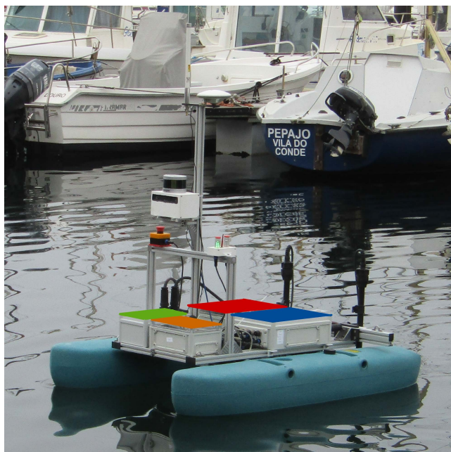
FIGURE 1. The SENSE full configuration mount. Green, orange, blue and red squares are the energy, localization, perception and navigation modules, respectively.
