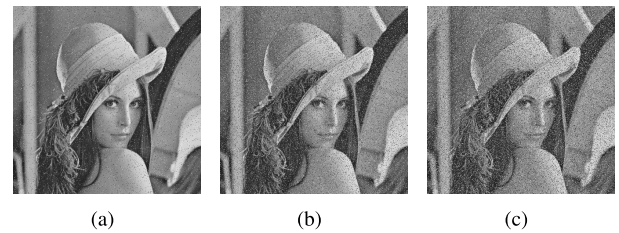
FIGURE 16. Image anti-noise test. (a) Decrypted image with 5% noise. (b) Decrypted image with 15%. (c) Decrypted image with 25%.
