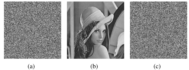
FIGURE 15. Key sensitive analysis diagram. (a) Cipher-image. (b) Use the correct key to decrypt. (c) Decrypt using a key that has been changed by one bit.
