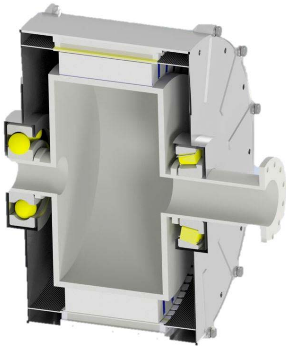
FIGURE 7. Half-section of a sketch of a electric motor with direct-liquid-cooled tooth coils, a spoke magnet type rotor and a hollow shaft.
